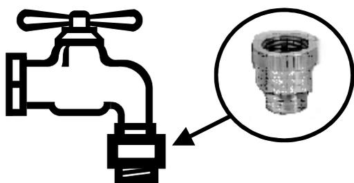
Another method of preventing backflow with a garden hose is using a device known as a vacuum breaker. Vacuum breakers are inexpensive devices that can be screwed onto your outside faucet. These devices will prevent contaminants from being siphoned back into your plumbing and the public water system.
