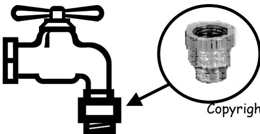
Another method of preventing backflow with a garden hose is using a device known as a vacuum breaker. Vacuum breakers are inexpensive devices that can be screwed onto your outside faucet. These devices will prevent
